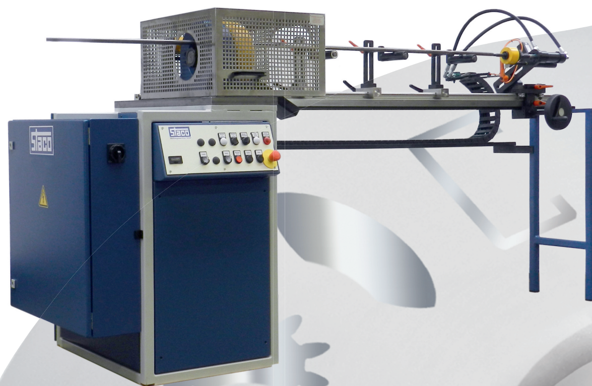
Semi-automatic AMH4 - hydraulic cutting machine for material with a diameter of up to 30 mm. The length is adjusted via a handwheel.
